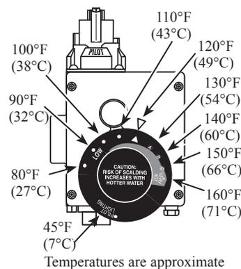
The illustration at the left details the approximate water temperature for each mark on the Gas Control (Thermostat) Temperature Dial.
